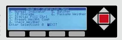
the Mode of Operation. You can then access other ID-related set-up screen like ID Counter by answering follow-up questions. The JAC 350 does the rest by configuring the normal operating screens such that each operational step associated with ID Storage is located within the four soft keys.
